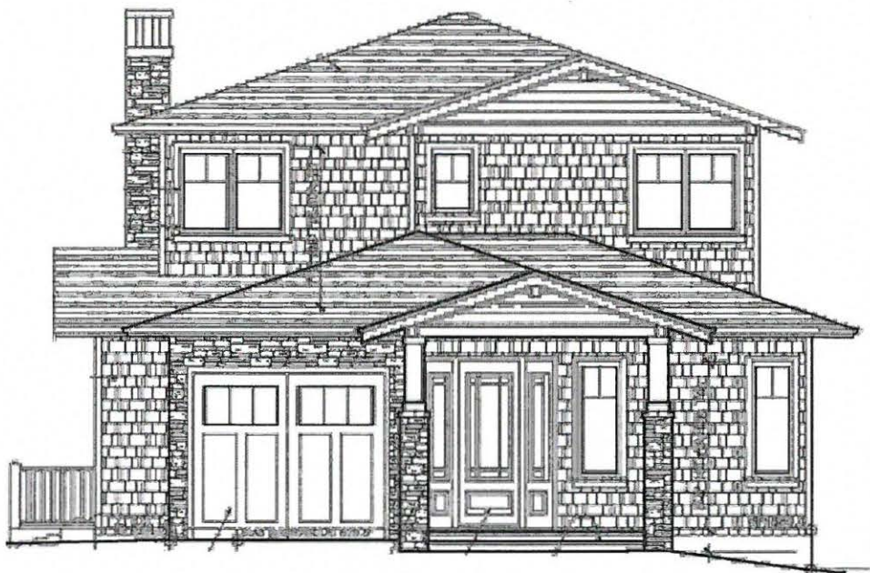
Revised Front Elevation - with shingles and stone in lieu of stucco
