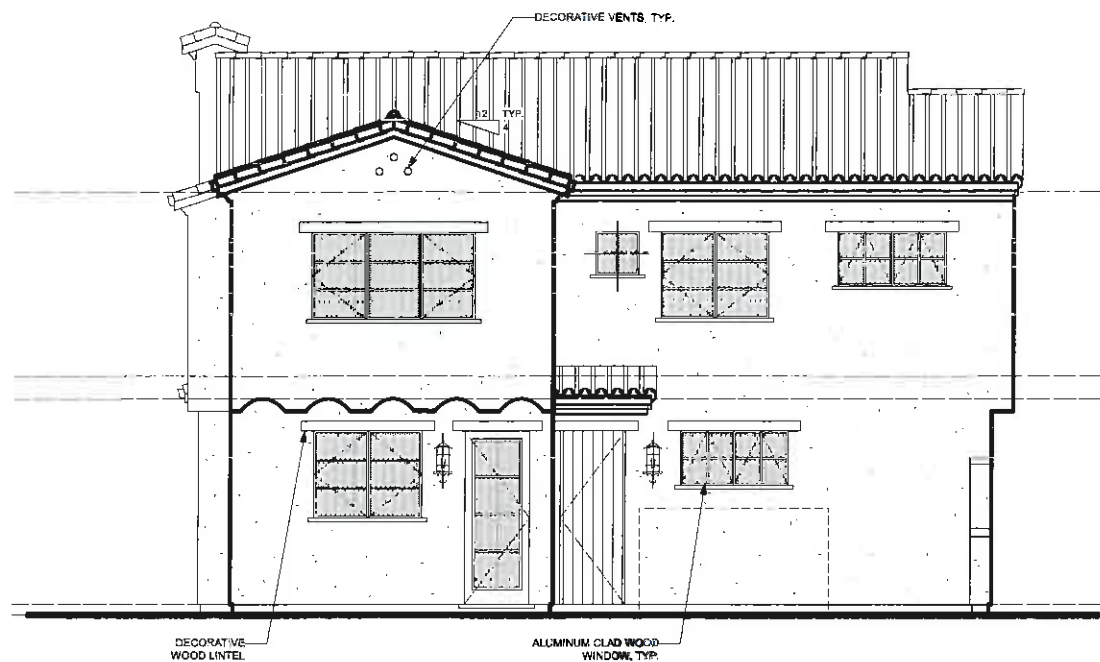
4 UNIT 4 - EAST ELEVATION SCALE: 1/4" = 1'-0"
