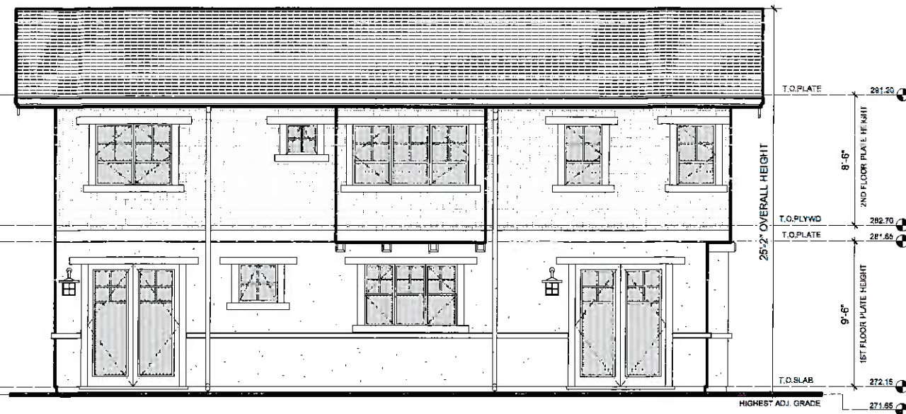
3 UNIT 1 - NORTH (REAR) ELEVATION SCALE: 1/4" = 1'-0"
